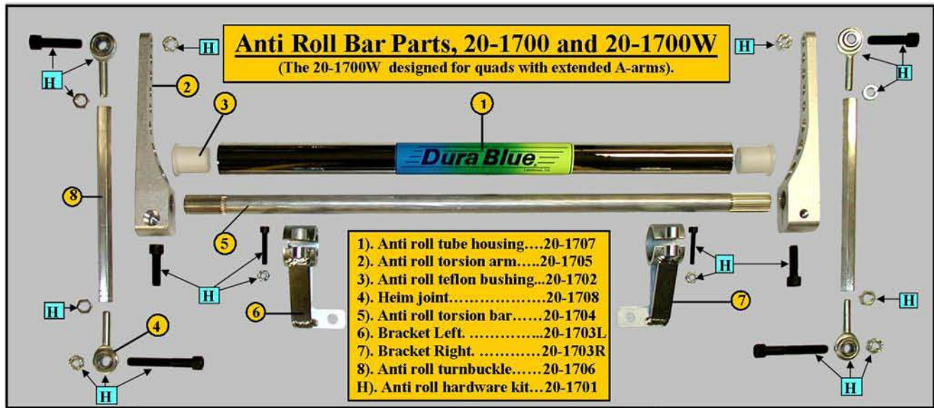
(Diagram 1) Parts break down, 20-1700 and 20-1700W
