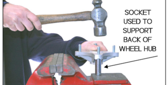
THE RIGHT WAY TO REMOVE STUDS
